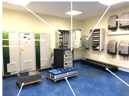
Li-ion storage 7.2kWh; 48V/150Ah Supercapacitors 0.294kWh; 300V/23,5F
